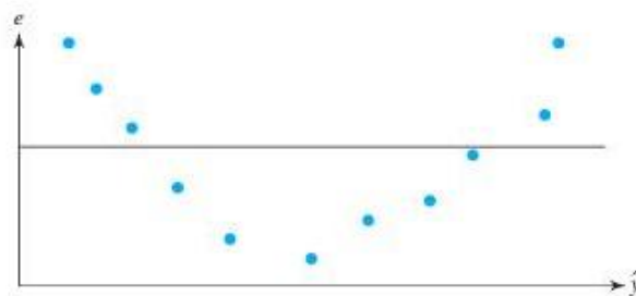
Figure 6.6 Systematic Curvature in a Residual Plot
