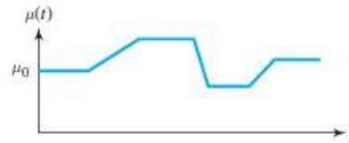
Figure 5.1 Typical Drift in a Process Mean over Time
