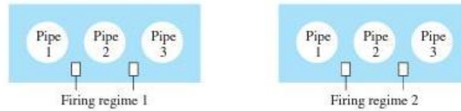
Figure 1.8 Experimental Setup for the Sewer Pipe Experiment
